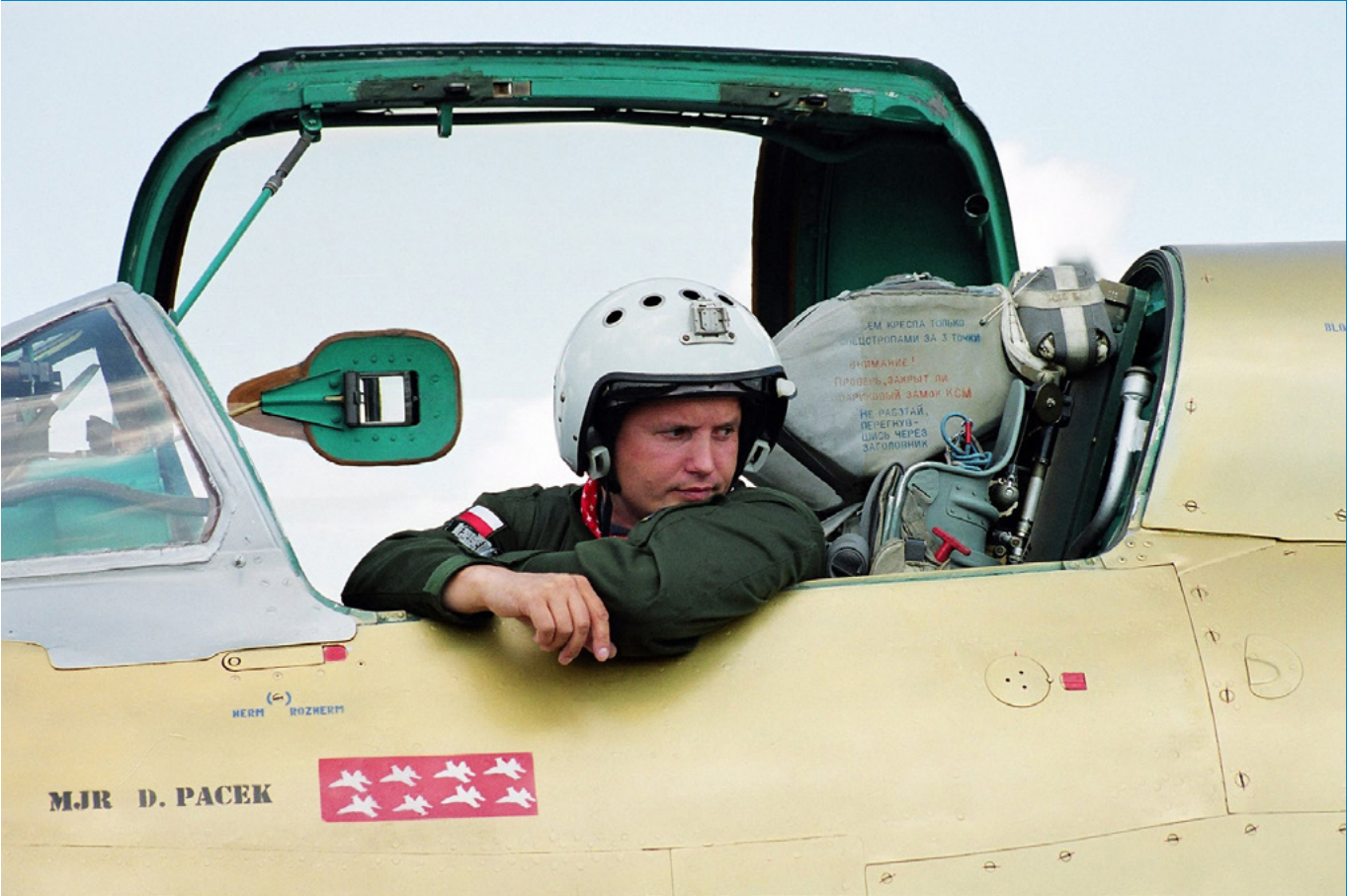
Canopy hinged to starboard. Rear view periscope mirror is visible. Commander of the 10 th Aviation Regiment in Łask mjr Dariusz Pacek sitting in the cockpit. (Dariusz Karnas)
