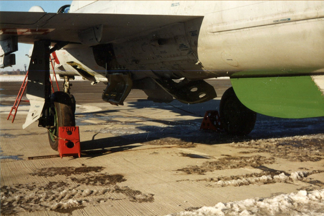
Main wheel leg and rear air brake in open position. (Dariusz Karnas)
