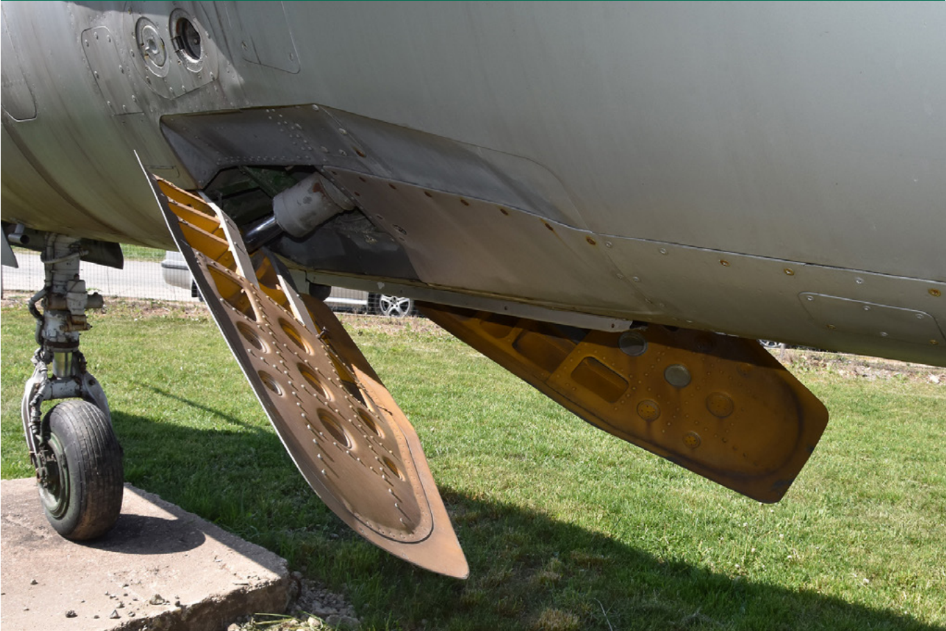
Front air brakes (both sides) in open position. (Dariusz Karnas)
