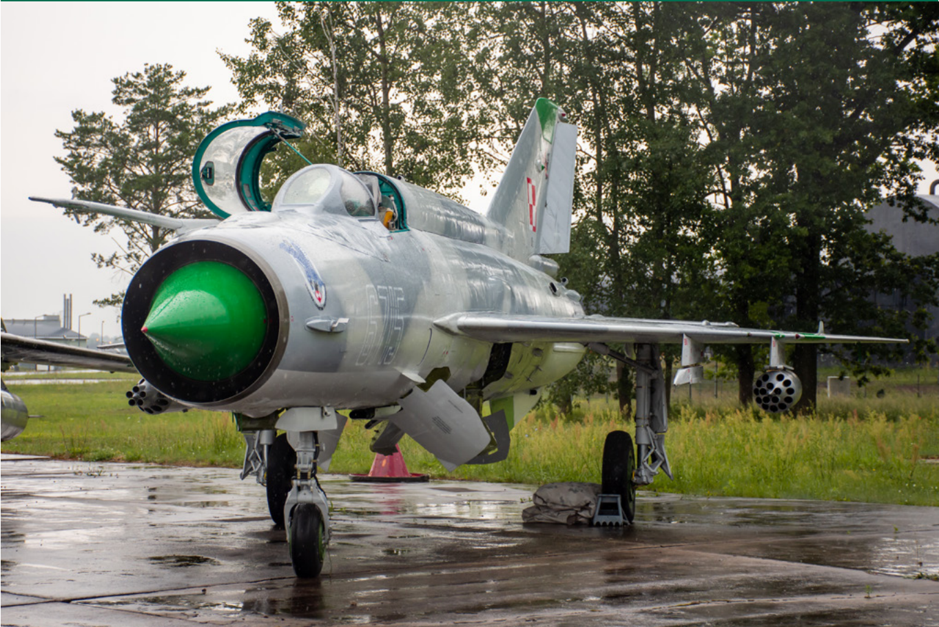
MiG-21MF “6715” s/n 96715, 10 th Aviation Regiment in grey/grey camouflage on an apron. Canopy hinged to starboard is visible. Front, and rear airbrakes in open position. (Leszek Jóźwik)
