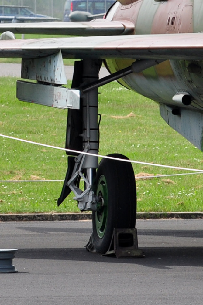
Main wheel legs and wing pylon with launch rail. (Dariusz Karnas)
