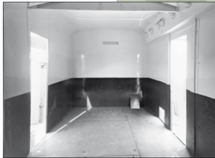
The inside of a typical box-body, with the lower half in a dark scuff-resistant colour, and the upper half pale to maximise light. (TM 1667/B/4)
