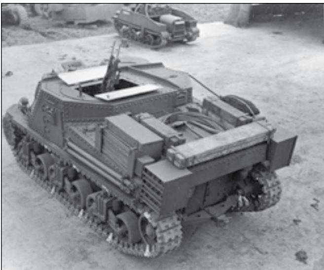
A Grant ARV showing the inside of the hatch covers still in White. (TM 2878/A/6)
